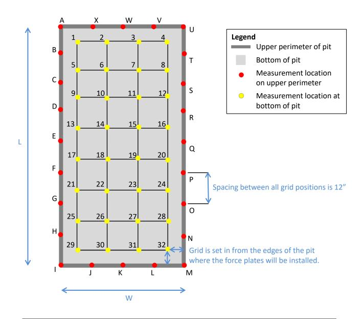
Position a laser level on the surrounding floor. Measure the depth from the plane to the floor along the upper perimeter of the pit on 12" increments and at every corner. Identify the high spot.
