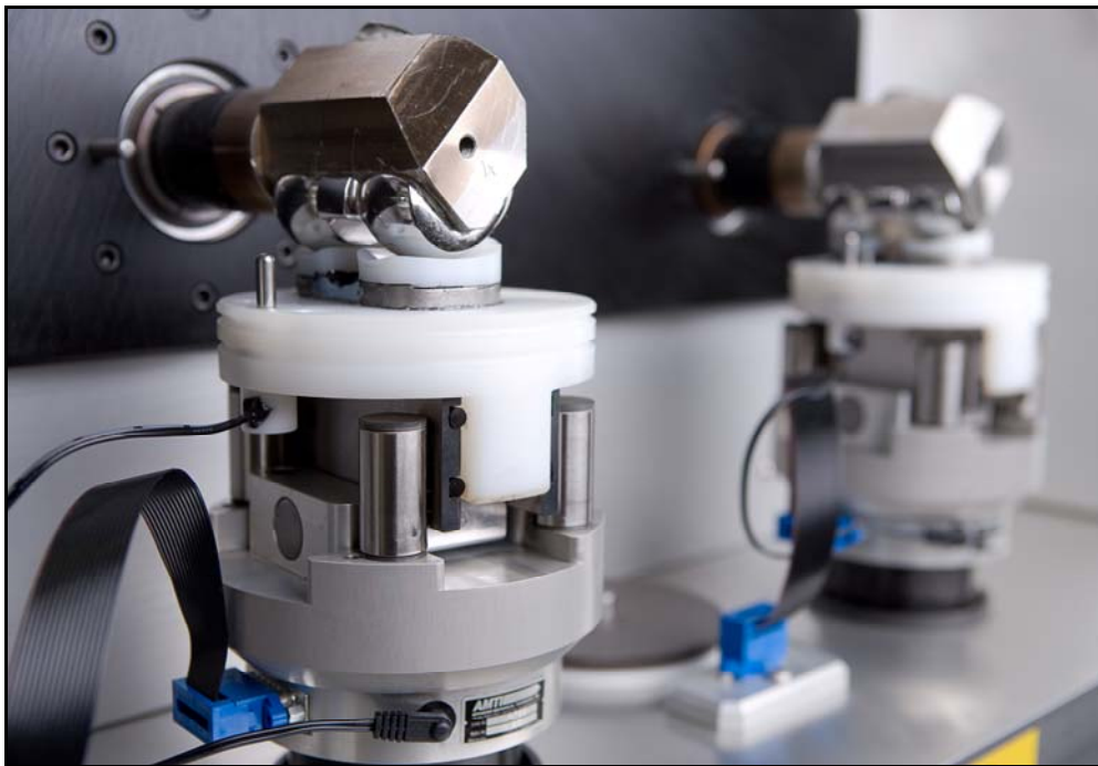
Two of the ADL Knee Simulator's six stations
